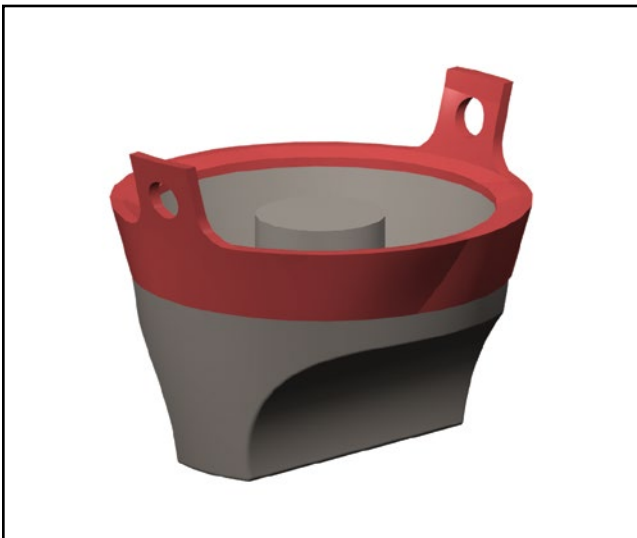
3-D model of conductive silicone custom masking for appliance knob allows part to be masked and hung from integrated tabs.
